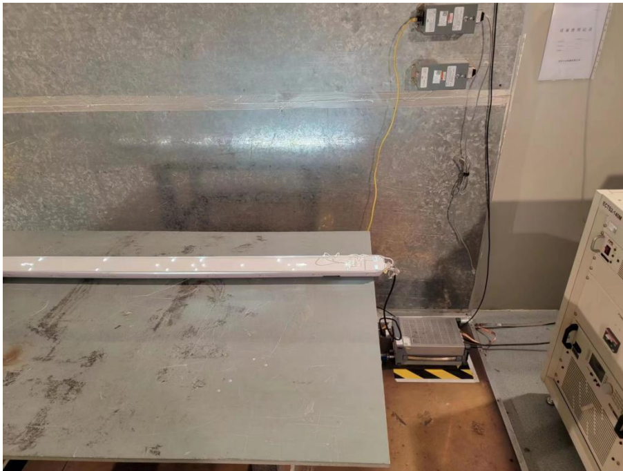
Photograph 2: Set-up for measurement of disturbance voltage
