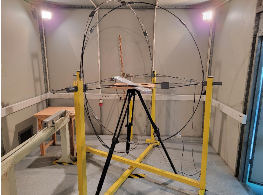
Photograph 4: Set-up for measurement of radiated electromagnetic disturbances (30-1000 MHz)
