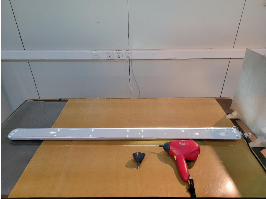
Photograph 5: Set-up for immunity test of ESD
