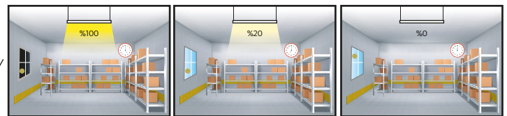
Once the ambient illumination level reaches 700 lux, the Led Tube will automatically switch off.
