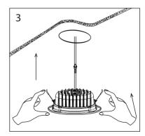
Energize the luminaire by plugging in the led downlight and driver output socket. After making sure that the product is working, lift the springs on the downlight backwards and release it freely into the space opening to the ceiling.
