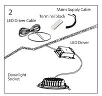
Connect the mains supply cable and Led driver output cable with a suitable terminal block in accordance with the cable colors.
